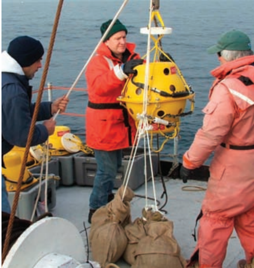
The buoy, above, is used to help anchor the LNG vessel and its network of pipelines to the mainland.
